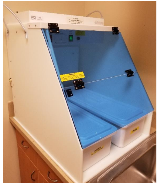
Filtration Control System (PCI Air Control recommended)
